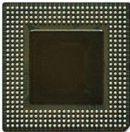
Bottom view of an Intel Embedded Pentium MMX, showing the blob of solder
